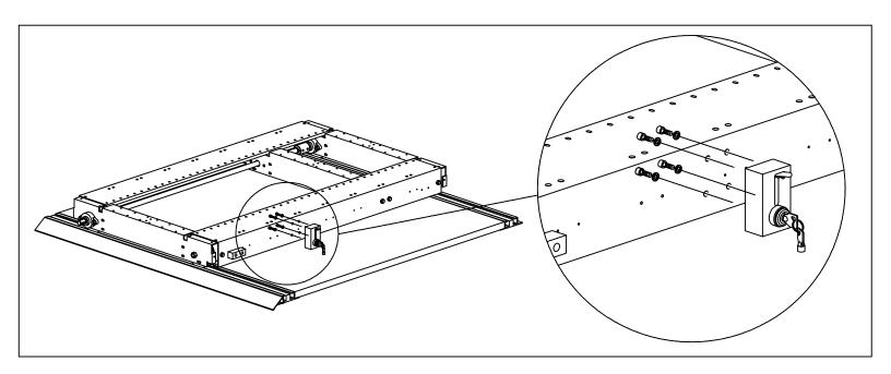
After Floor Lock is mounted to the vertical surface of the skirt, compress all mobile systems to the closed position. Let the 1/2" bolt of the floor lock drop to the deck panels of the mobile 1000 system. Draw a circle around the perimeter of the bolt. Move the carriage out of the way and drill a hole using a 1" diameter spade bit (not provided).
