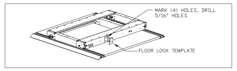
Using the (4)  $1/4-20 \times 5/8$ " Socket Head Cap Screws and (4) 1/4" Flat Washers, secure the floor lock to the skirt. Tighten the Cap Screws with the supplied 3/16" x 6" T-handle allen wrench.
