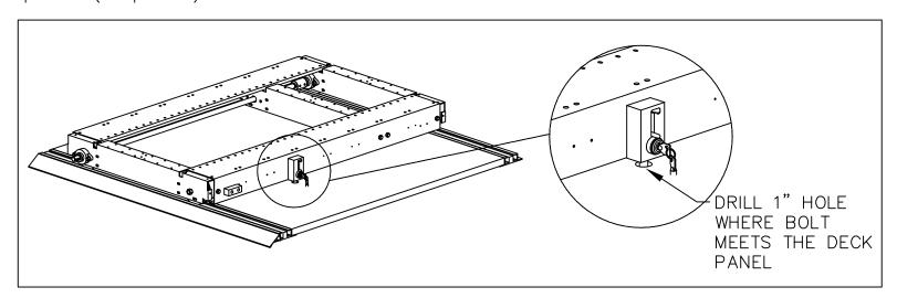
The final step is to install the Floor Lock Plate over the 1" drilled hole in the deck panel. The Floor Lock Plate is screwed to the deck panels using (4) #8 x 5/8" Wood Screws found in hardware bag 913050. Once complete verify that the floor lock is operating properly.
